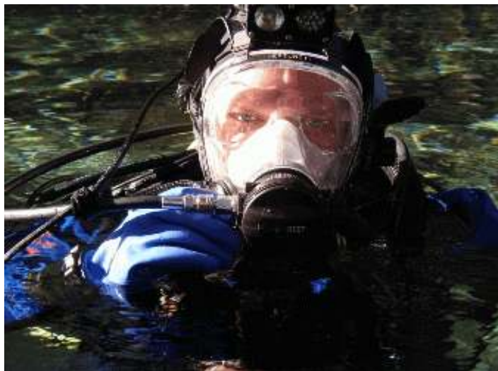
A Full Face Mask, drysuit with sealed gloves, integrated communications and light system.
