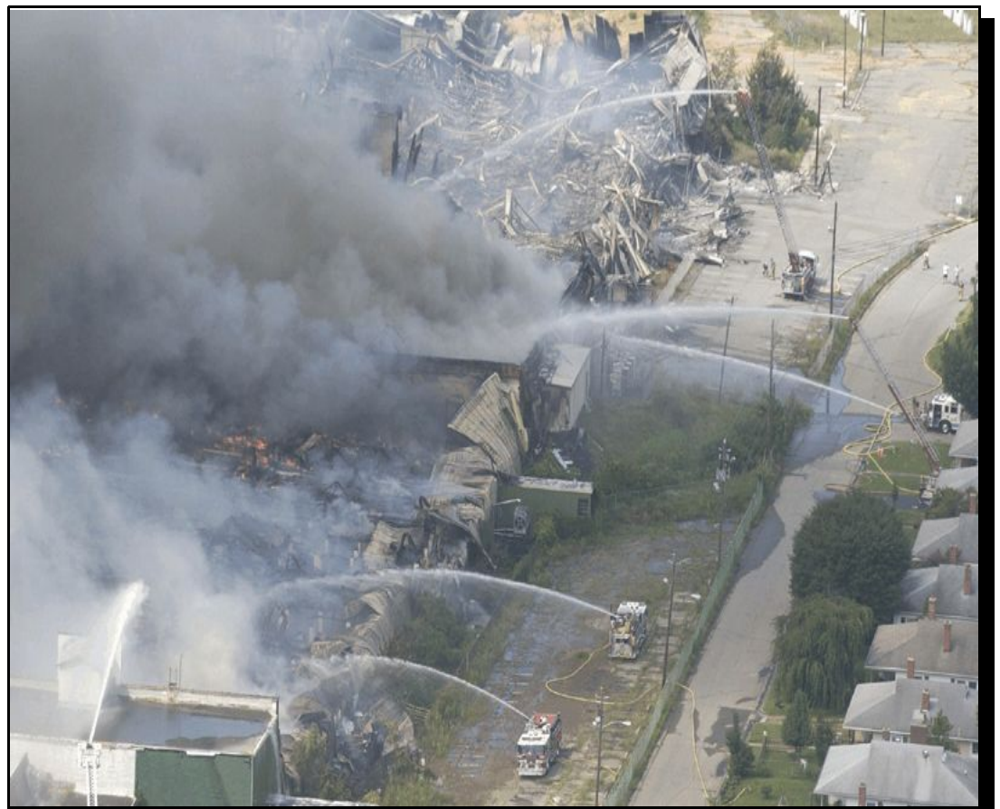
FIGURE 4 - Some defensive operations with exposure protection can easily require rates into the thousands of gpm. If the NFF for an exposure seems too low or isn't working, crank it up. (Beacon fire, Swannanoa, 2003. One structure suffered damage to vinyl siding at almost 200' away)
